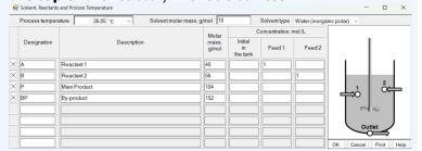
Next, enter the reaction details for both the main and side reactions, and update the corresponding kinetic data.
