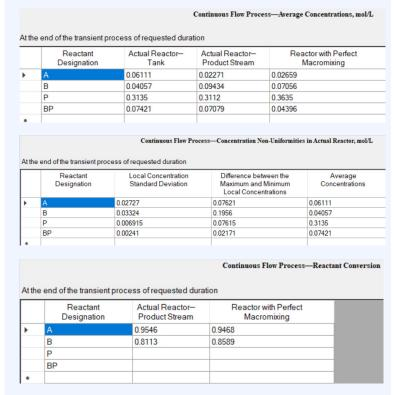
Reactant A achieved a high conversion of 0.95, slightly above the ideal 0.94, indicating efficient local micro-mixing. In contrast, Reactant B showed a lower conversion of 0.81 vs. the ideal 0.86, likely due to poor flow distribution or dead zones.
