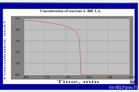
The duration of the cooling stage is about 5.3 minutes, and the total reaction time is about 10 minutes.
