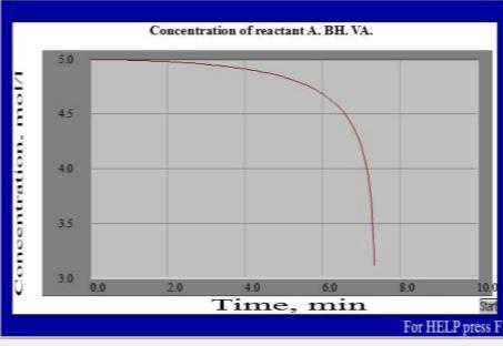
Based on these graphs the *first stage duration* is taken to be limited by 4.5 minutes from the start of the process and initial parameters of the second stage are 35°C and 4.85 mole/liter, respectively.
