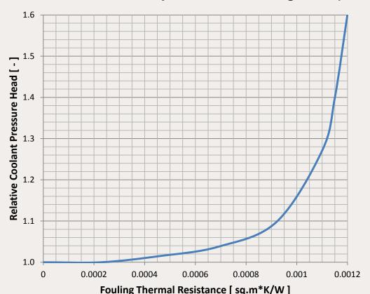
cooling and hence is setting the condition for the beginning of a runaway regime starting from the fouling thermal resistance  $\sim$ 0.001 m<sup>2</sup>\*K/W (for pure service water used as a coolant it corresponds to deposit layers with ~2mm thickness). Thus the VisiMix® enables to define a criterion setting an upper limit for the process stoppage.
