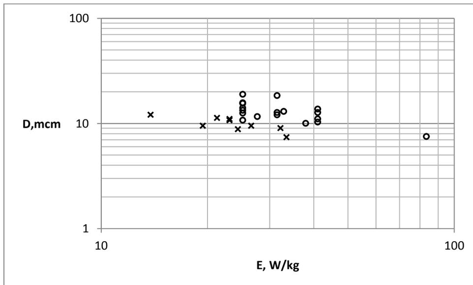
Figure 3. Influence of width of radial slots in stator on mean drop size. Stabilizer –Tween, 3%.
