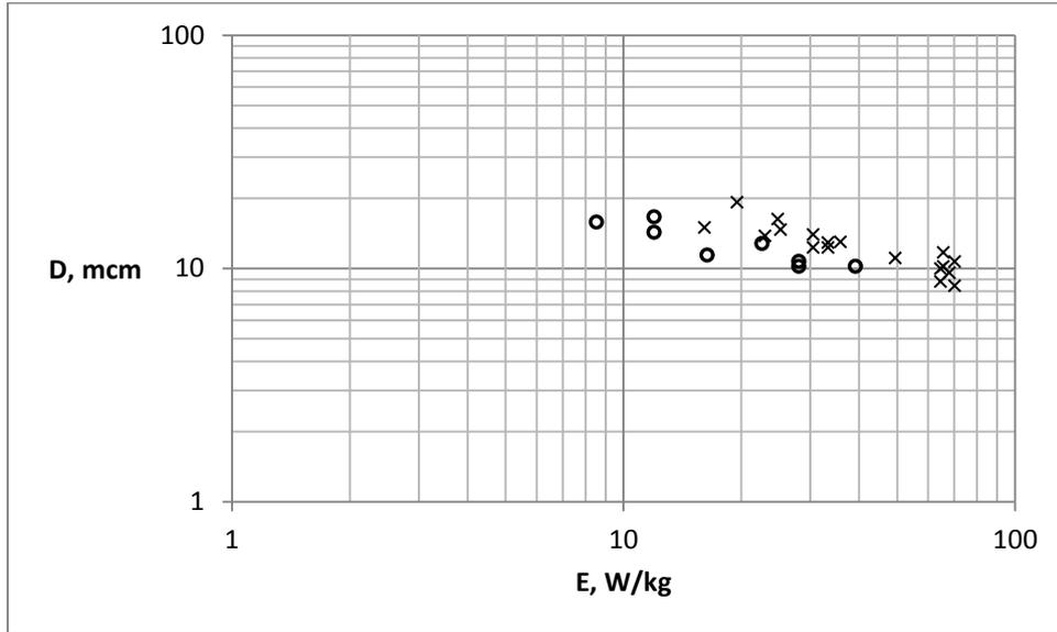
Figure 4. Influence of width of radial slots in stator on mean drop size. Stabilizer –Tween, 3%.
