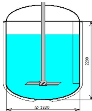
*Figure 2. The diagram of the stirred reactor*
