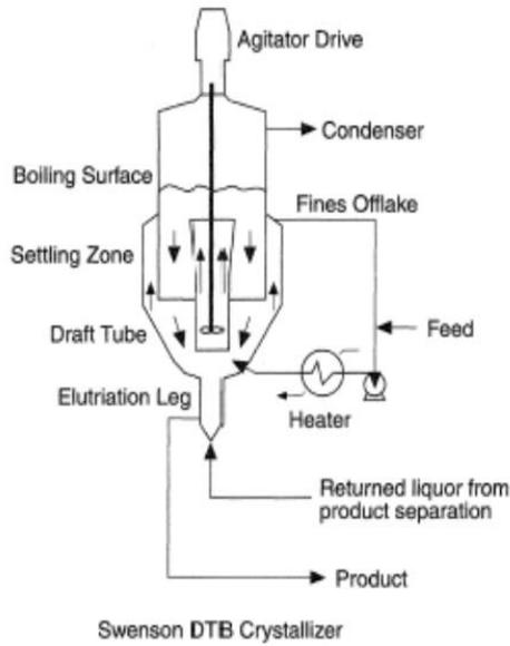
*Figure 15. Crystallizer with a Draft Tube*
