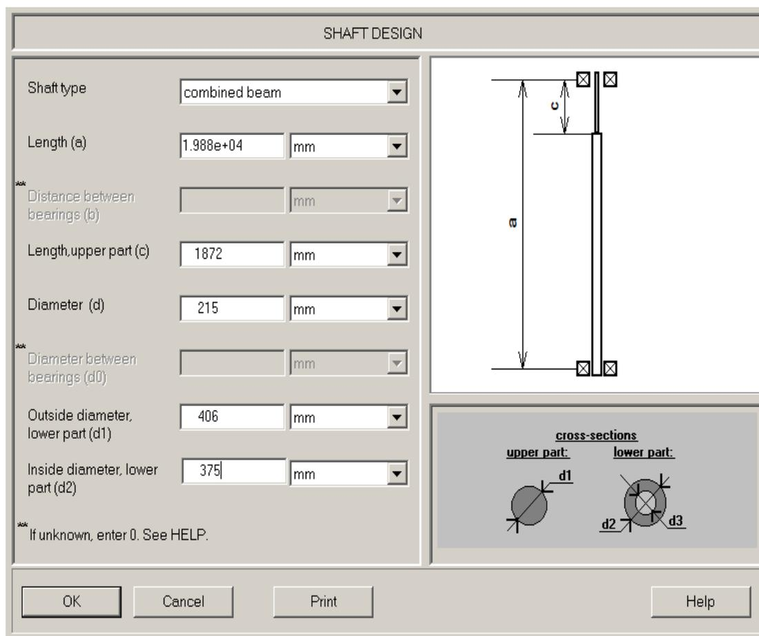
**Figure 20. The VisiMix® Model of the Modified Shaft**
