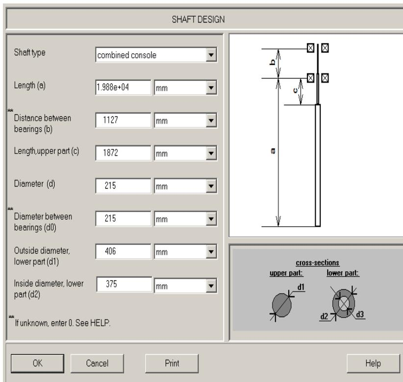
**Figure 17. The VisiMix® Model of the Shaft**
