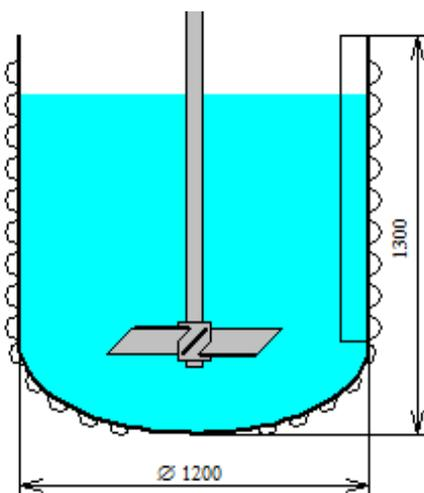
Figure 13. The diagram of the stirred reactor (Example 2)
