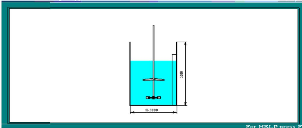
Figure 9. Scheme of the tank with impellers.
