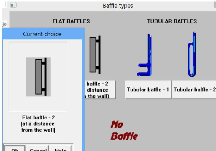
Figure 3. Graphic menu for selection of baffles (fragment).
