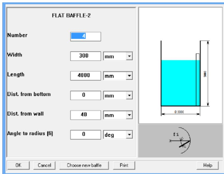
Figure 4. Entering data for the baffles.
