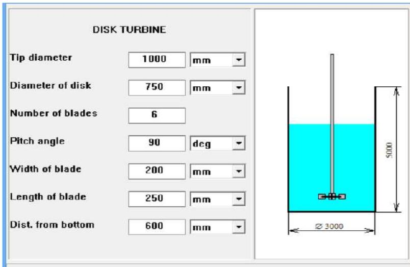
Figure 7. Entering the Impeller 1 - disc turbine.
