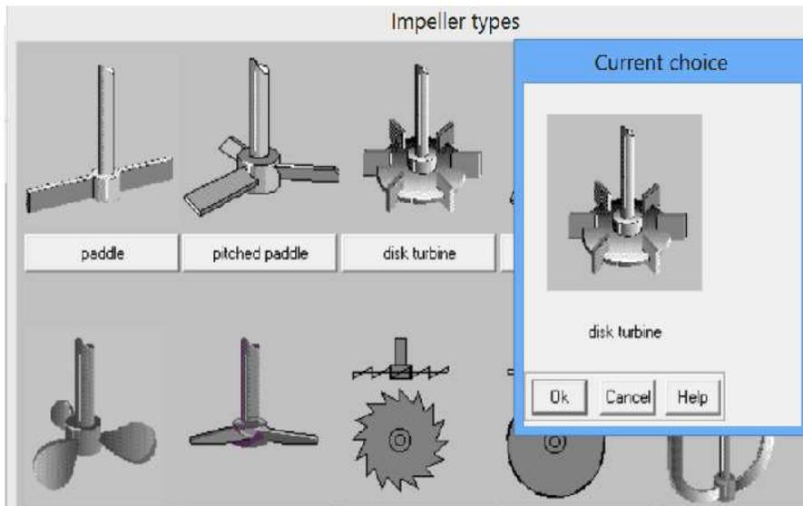
Figure 6. Graphic menu of impellers (fragment).
